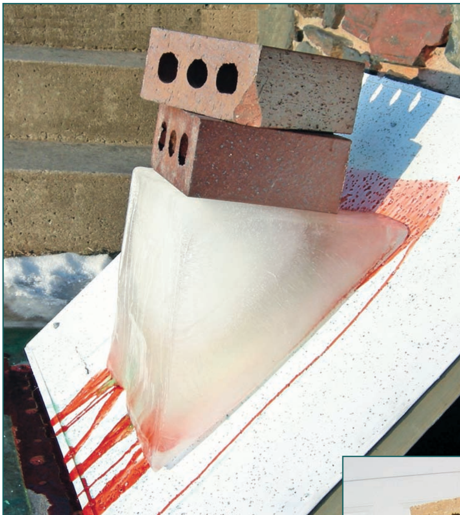
Photo 11 – Meltwater (dyed here for clarity) flows under the block without moving the block.
