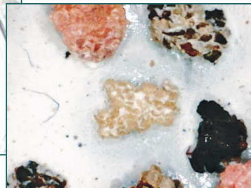
Photo 5 – Aggregate set in energy-saving white reflective base coat.
