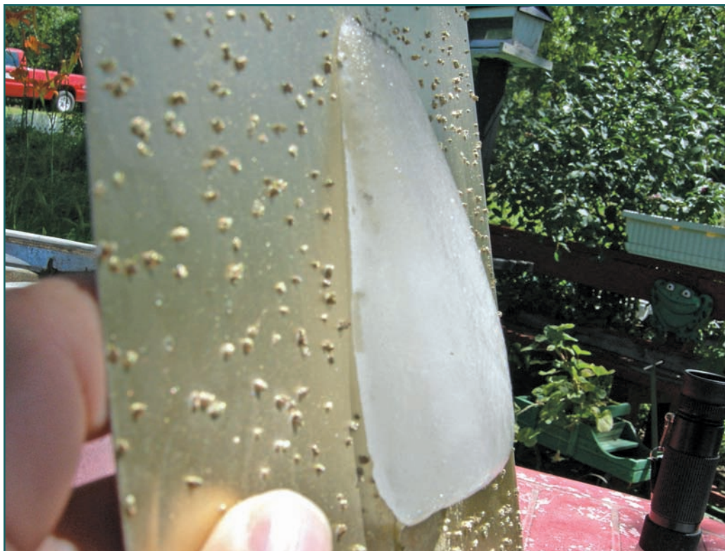
Photo 13 – Demonstration of aged ice block on sample in nearly vertical position.
