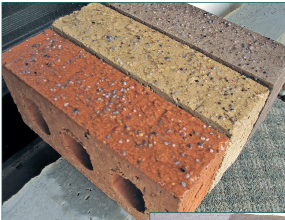
Photo 9 – SR coating sample on brick.
