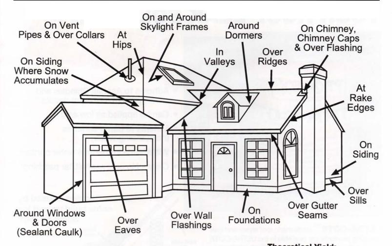
DYNA-SEAL is recommended for joints and seams wherever dissimilar materials meet.
